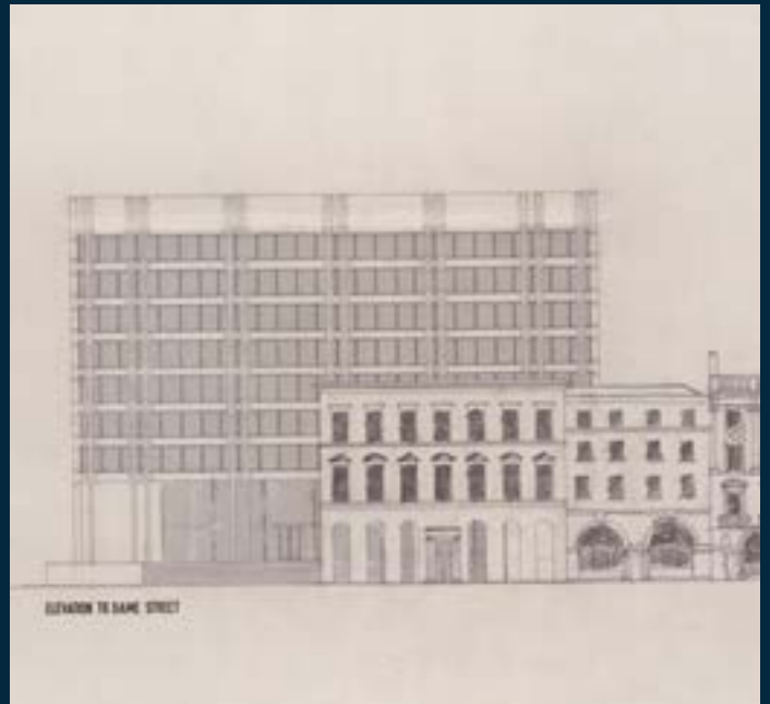
Proposed front elevation plan of the Dame Street Offices featuring 7 floors, and including the façade of Commercial Buildings, 1970.
